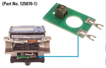
Combine the External Power Module and the Pulse Access Module to provide external power capabilities to a FLOMEC® Electronic Digital Meter.
